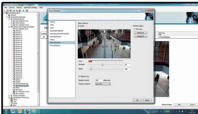
Performance-enhanced, built-in motion detection lowers memory and central processing unit (CPU) consumption even when additional cameras are added. Hardware is optimized by detecting motion on key frames or on a specific part of the video in regular quality or lower video resolution.
